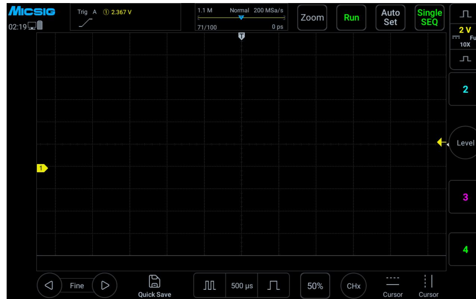
Figure 12-14 Single trigger segmented storage
