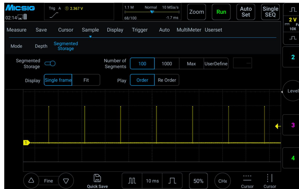
Figure 12-11 Segmented storage waveform acquisition
